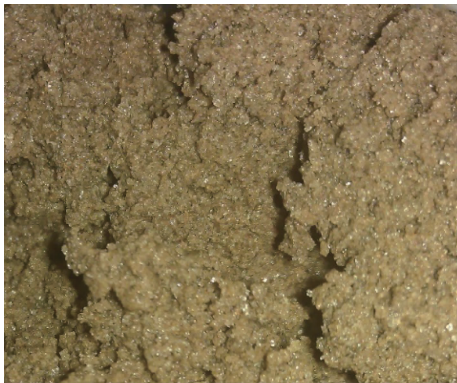
图 1 氯盐渍土样 Fig. 1 Chloride saline soil sample
